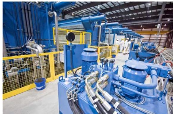
**Fig. 2:** membrane type filter presses
